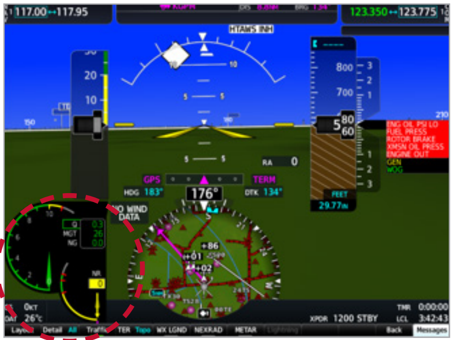
Power Situation Indicator.
